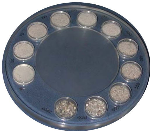
A sampler showing grains sorted from silt to very coarse sand.
